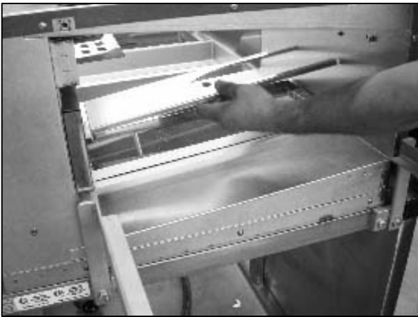
22. Lift up on the outside end of the lower air duct panel.
